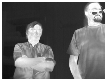
Figure 4: IR image obtained from 1024 x 768 / 17 \mu\text{m} sensor
